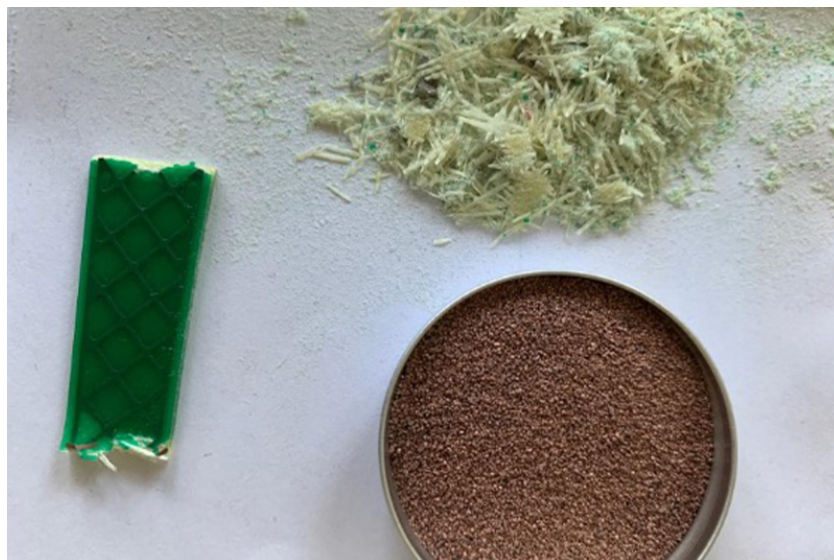
Predattec's system processes complex e-waste without chemicals or heat — powering a cleaner circular economy. The picture above showcases materials recovered from a PCB: copper, fiberglass, and epoxy dust.
